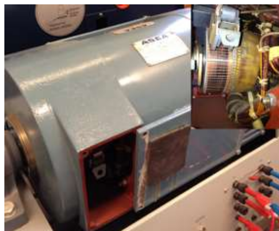
Figure 28 An example of a DC-machine with a commutator and brushes shown inset in the top right corner.
