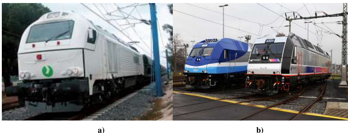
Figure 4 a) Vossloh EURODual for freight purposes comes with three different diesel options: 700 kW, 1400kW and 2800 kW. Electric traction 5000 kW. b) Bombardier ALP-45DP for freight and passenger service (Line between New Jersey and Montréal). Electric traction 4000 kW, diesel traction 3134 kW.
