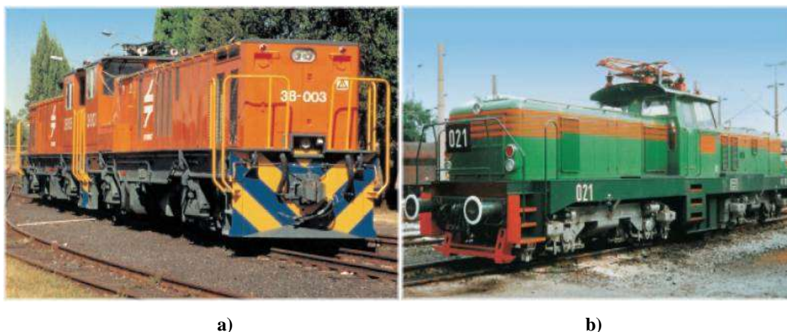
Figure 5 a) Class 38 traction power 1500/780 kW b) ED1600 traction power 1600/560 kW
