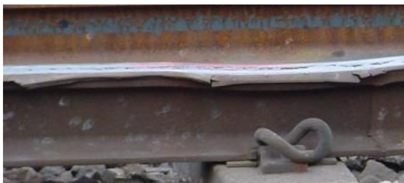
Figure 2 – Rail Contact Fatigue & Deformation
